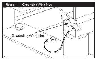
Generally, connecting a No. 12 AWG (American Wire Gauge) stranded copper wire to the grounding wing nut and to an earth-driven copper or brass grounding rod (electrode) provides adequate protection against electrical shock. Be careful to keep the grounding wire attached after connecting the stranded copper wire. However, local codes may vary widely. Consult with a local electrician for grounding requirements in your area.
